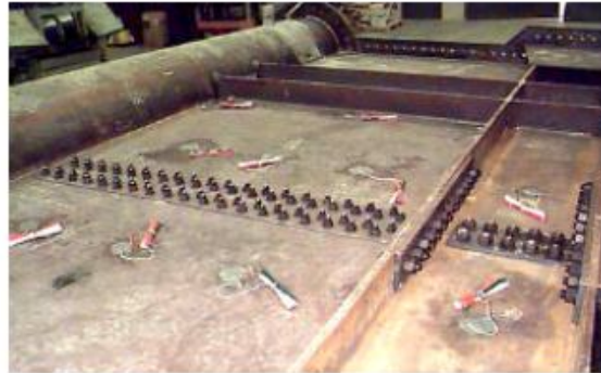
Components of the tested system and bolted splice
